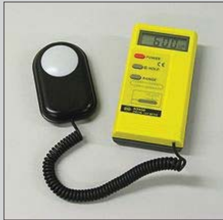
A lux meter for measuring illuminances in work places.
