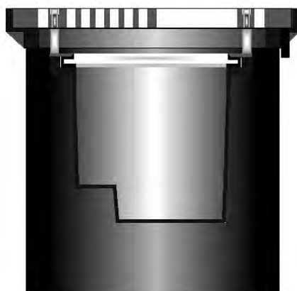
Complete buried upright with IP 69 Projector - sectional view
