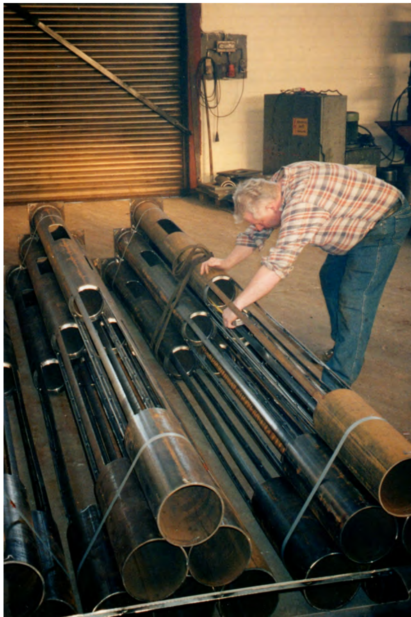
Tubes ready for hot dip galvanizing
