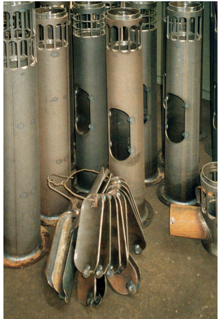
Bollard fixtures , ready for being hot dip galvanized.
