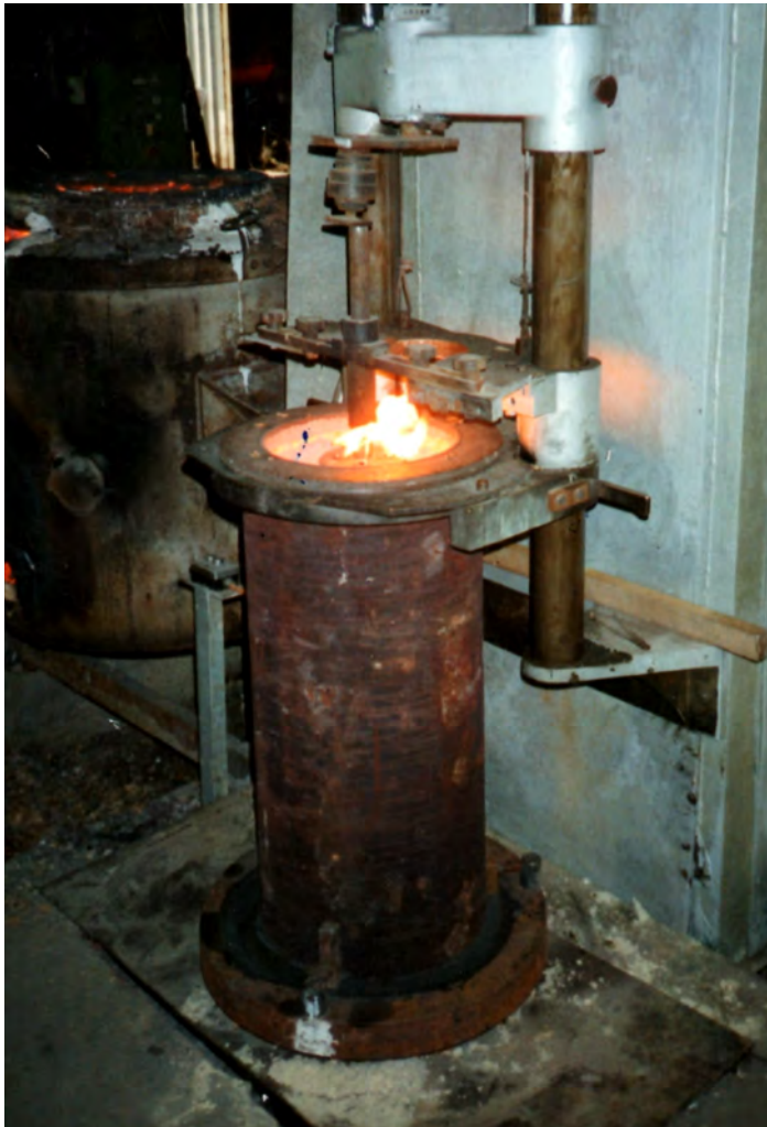
Aluminum casting: Tool for base of bollards
