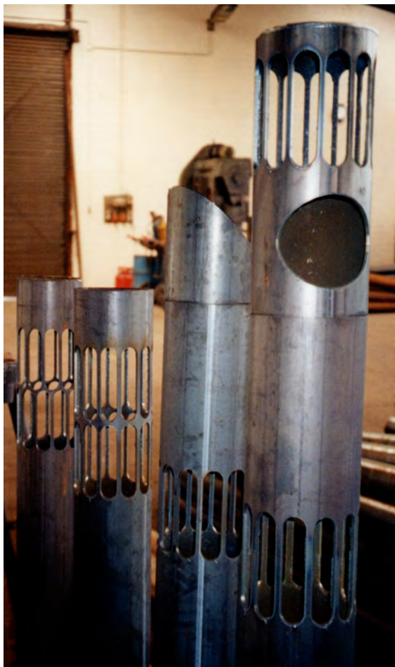
Cut steel tubes prepared to be welded
