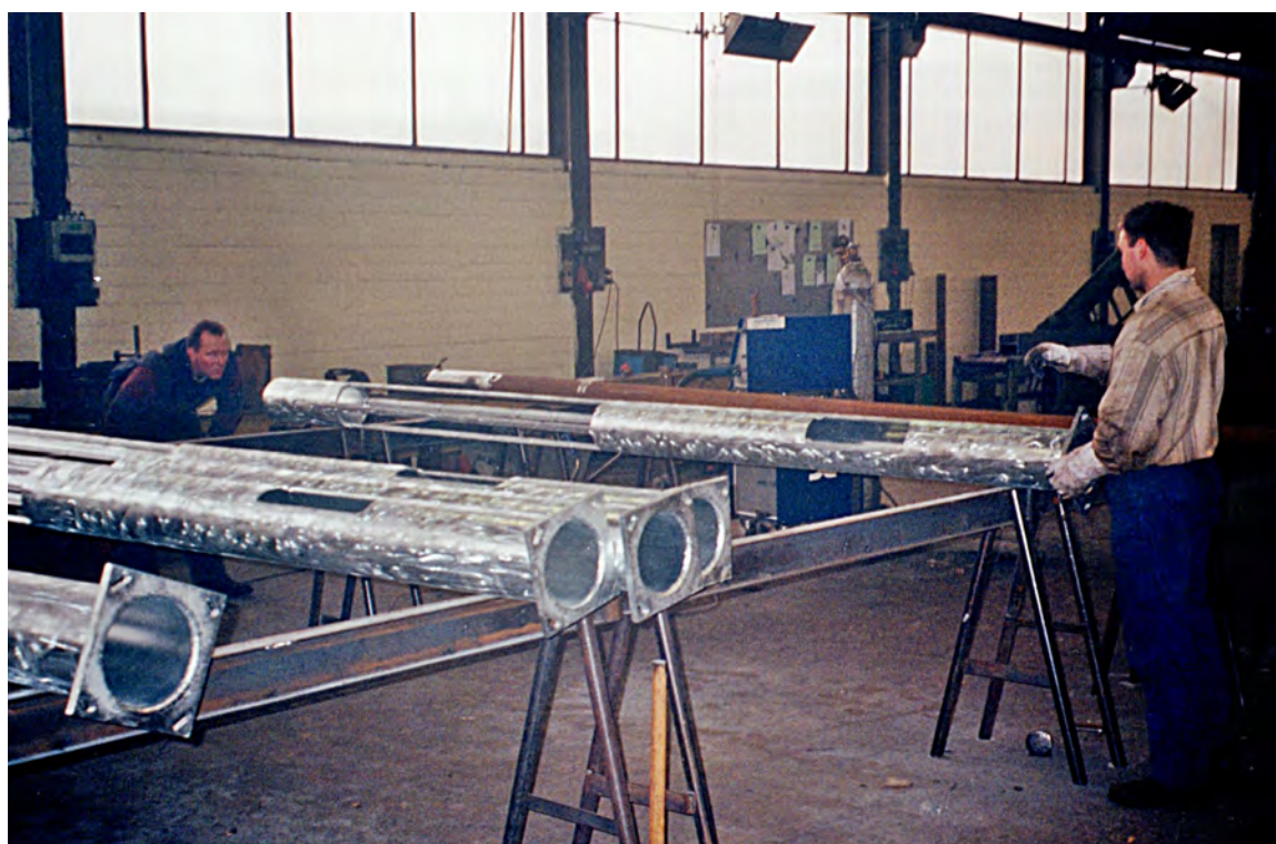
Tubes ready for hot dip galvanizing
